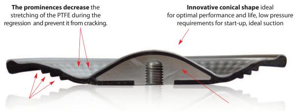
Innovative diaphragm support side, offers flexibility, long life and protects from cavitation **Special internal plate** supports your diaphragm in every movement
