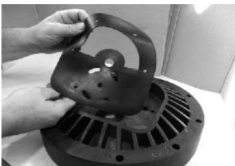
Step 4 Mount central block with air chambers
