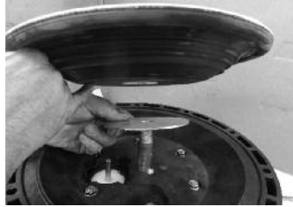
Step 2 Insert into the shaft the piston inner and the diaphragm and mount.
