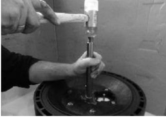
Step 1 Insert shaft into bearings in which you have put already PG MOLYKOTE 21
