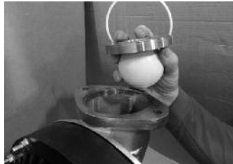
Step 5 Install ball valves, ball seats, o-rings
