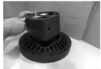
Step 3 Install flanges into the air chambers
