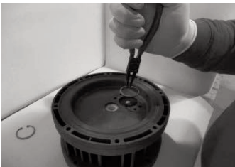
Step 1 - Step 2 We remove the safeties (step 1) and push from the one side the air control unit towards the outer part (step 2)
