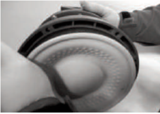
Step 4 Detach the diaphragm from the central block by hand and untie it with a left rotation.
