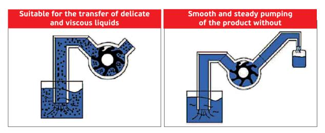
Up to 75.000 cps, even with solid suspension, without any wear out or damage.
