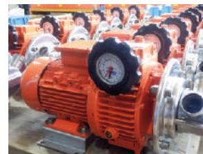
As an option AD flexible impeller pumps are available with a variable speed drive that allows the flow rate to be finely adjusted by changing the RPM of the pump. This also allows to achieve a soft pumping action to handle delicate and highly viscous liquids
