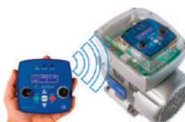
Some models have a built-in IP65 rated motor-inverter with wireless remote control. This allows to directly adjust the RPM of the motor, reducing the weight and size of the pump assembly as it doesn't require a mechanical gear unit
