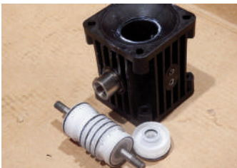
Step 7 Remove the air control unit from the central block
