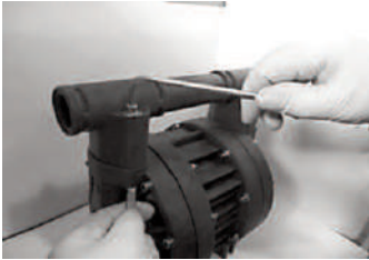
Step 1 Remove the discharge manifold by untying the screws in X formulation
