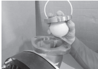
Step 5 Install ball valves, ball seats, o-rings
