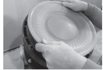
Step 3 Repeat same process also for the other diaphragm after having installed the pump housing first
