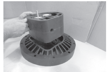
Step 3 Install flanges into the air chambers
