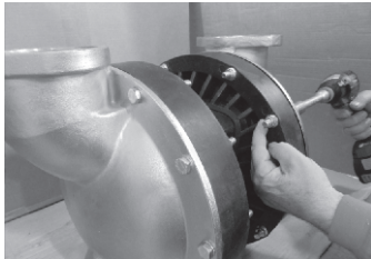
Step 4 Install also second pump housing and mount on
