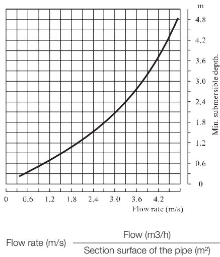
Suggested suction pipe submersible depth vs flow rate
