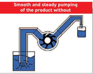
pressure from the spikes (even flow rate is ideal for filling, dosing or filtration)
