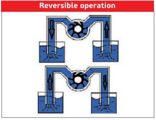
The pump can work in both the 2 directions of operation with interchange of the flow of the liquid inside the network without a problem, as many times as we want with a simple interchange of the motor direction.
